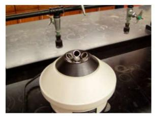
water if necessary (do NOT dilute another solution with tap water; instead, place it in its own slot and balance the centrifuge). If the centrifuge is not properly balanced, it is very easy to severely damage the centrifuge. If you understand the concept of vectors, you can balance the centrifuge with three test tubes as well; ask your instructor for more information.
