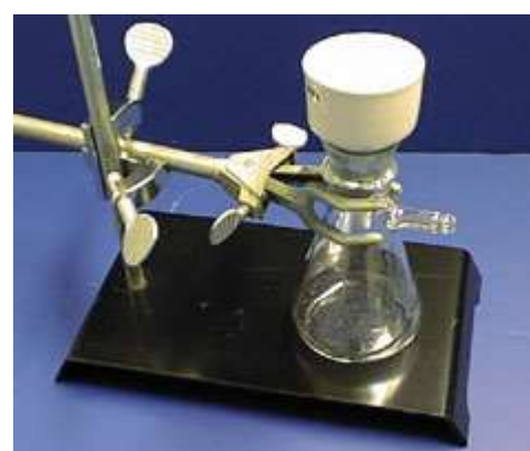
place the Buchner funnel on the adaptor
