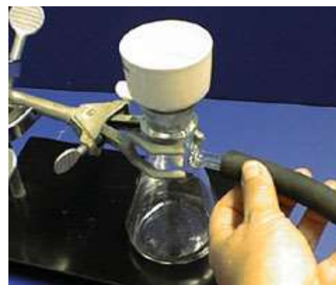
connect the side arm flask to a vacuum source - always use thick-walled tubing , since Tygon tubing will collapse under reduced pressure
