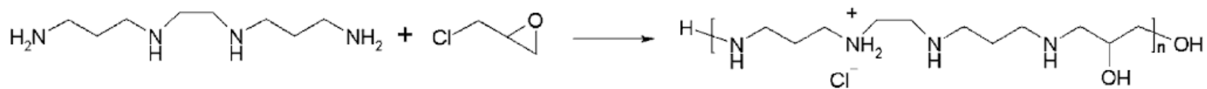
Fig. 3. PolyE-323 polymer synthesis scheme. The polymer is schematically depicted and the charge of the polymer is dependent on pH. PolyE-323 has a low degree of branching, which is not indicated in the schematic structure.
