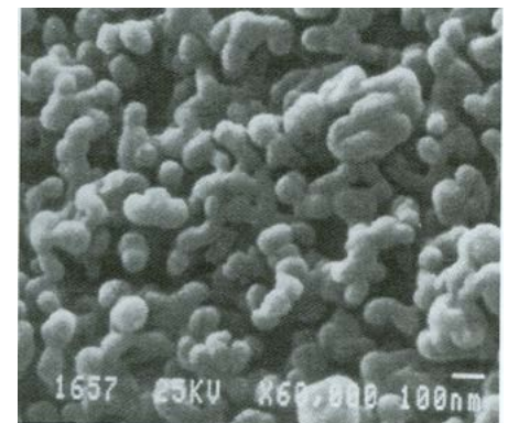
Close-up SEM of a typical silica gel surface showing pore structure.
