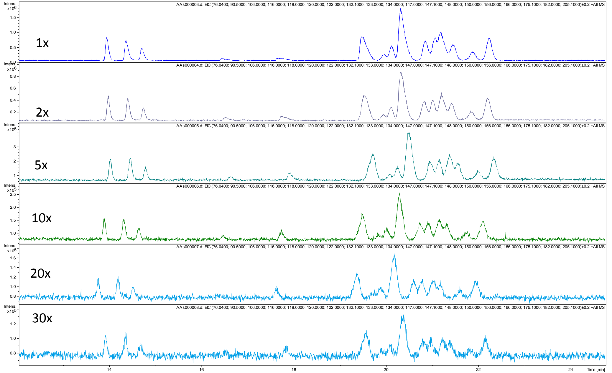
Aminosav keverék 1-30x hígításainak CZE-MS elemzése Minta (1x): Minta: 5 mM Gly, 8 mM Ala, 2.5 mM Ser, 2.5 mM Val, 5 mM Thr, 0.5 mM Cys, 0.5 mM Ile, 0.5 mM Leu, 2.5 mM Asn, 2.5 mM Asp, 0.5 mM Gln, 0.5 mM Lys, 0.5 mM Glu, 0.5 mM Met, 0.5 mM His, 0.5 mM Phe, 0.5 mM Arg, 0.5 mM Tyr, 2.5 mM Trp
